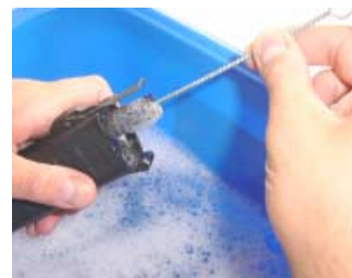
cleaning of the barrels and nozzles with soap water
